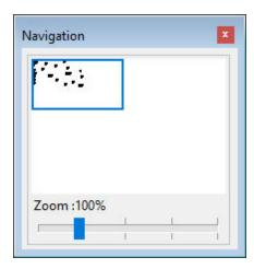
When the zoom percentage display is higher and the navigation square is smaller than the model, the blue navigation square can be dragged to specific areas of the model allowing a clearer view of the model's tables.
